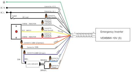
3. Emergency Solution with non-dimming LED driver (\* LED DRIVER INPUT POWER NOT GREATER THAN 8W)
