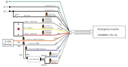
2. Emergency Solution with 0-10V LED driver, without using 0-10V dimmer (\* LED DRIVER INPUT POWER NOT GREATER THAN 50W)
