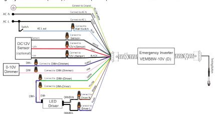
2. For luminaire with 0-10V LED driver, without using 0-10V dimmer (\* LED DRIVER INPUT POWER NOT GREATER THAN 60W) Emergency Inverter Dim+ (Green), Driver Dim- (Yellow) has to connect with LED driver DIM+ and DIM-
