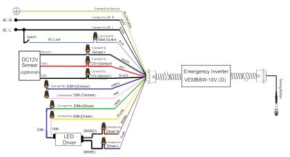
3. For luminaire with non-dimming LED driver (\* LED DRIVER INPUT POWER NOT GREATER THAN 8W)
