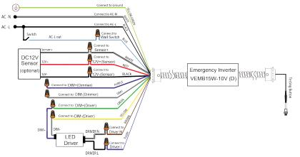
3. For luminaire with non-dimming LED driver (\* LED DRIVER INPUT POWER NOT GREATER THAN 15W)
